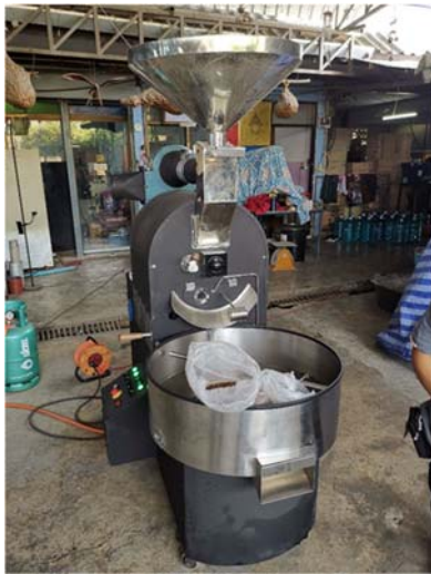
Fig. 4. shows the hardware system of the fully assembled coffee roaster.
