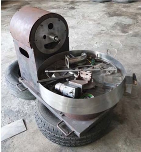
Fig. 3. shows the installation of roaster tank to the cooling rack.
